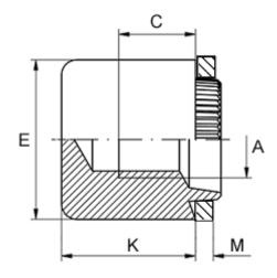
Female thread A = M8Height K = 12.0Min thread length C = 6.0Outer diameter E = 16.0Plate thickness = 3.8 to 4.0
